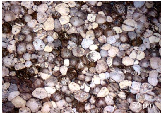
AM-SC1™ grain refined with AM-cast Average grain size 16 µm
