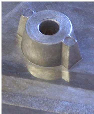
Figure 11a: As-cast surface of AM-HP-2 - surface roughness profiles on the body of the casting and the mirror finish surface
