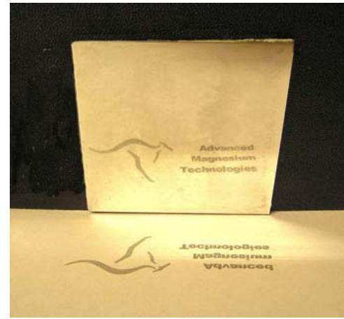
Figure 2. As-cast mirror finish on diecast AM-lite plate (top half of picture)
