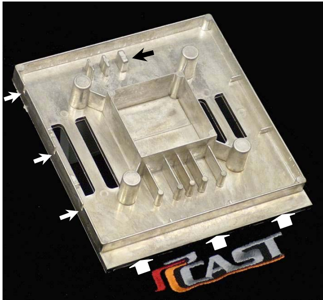
Figure 1. A part made in the new castability die in its as-cast condition. The 3 part fanned gate enters the casting from the lower part of the photograph.
