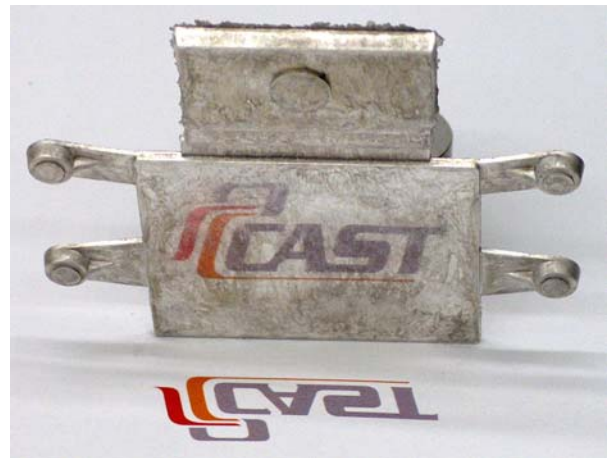
Figure 2. AM-HP2 part showing a high quality reflective surface finish in the as-cast condition (plate is 70 mm wide).
