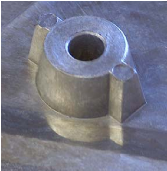
Figure 8: As-cast surface of AM-HP-2 - an example of the mirror finish achievable on the casting facing the polished section of the die.
