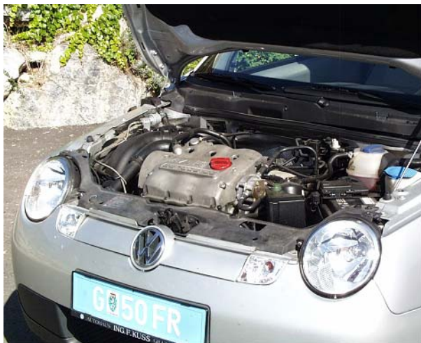
Figure 6. Genios LE turbo-diesel engine developed by AVL list utilizing sand cast AM-SC1 for the block
