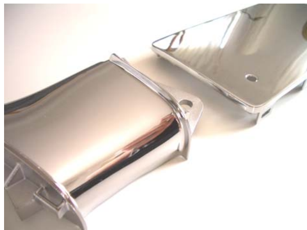
Figure 2. Automotive components diecast in AM-lite and electroplated using MacDermid's electroplating process
