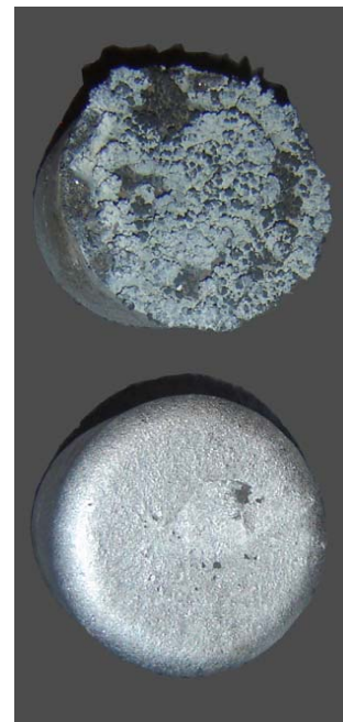
Figure 5. Comparison of oxidation of AZ91D (top) and AM-lite (bottom) solidified in air
